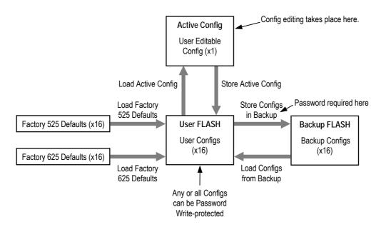
Figure 4.22: Configuration, Graphical Explanation.
